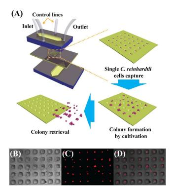
**Fig. 2** (A) The entire process for the high-throughput single cell capture, single cell based culture to form colonies, and retrieval of the produced colonies. (B) The bright field, (C) the fluorescence and (D) the merged images showing uniform single *C. reinhardtii* capture in the hemispherical perforated microwell structure.
