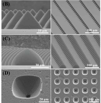
**Fig. 1** (A) Fabrication process of hemispherical perforated microwell structure. SEM images of a replicated PDMS from a Si wafer (B) after anisotropic wet etching and (C) aniso- and isotropic wet etching. (D) SEM image of a large-scale hemispherical perforated microwell structure.
