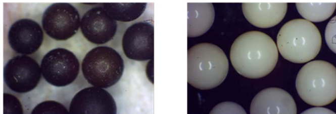
Figure 3: Amberlyst 46 images (x15) after and before all the experimental CPO deacidification tests
