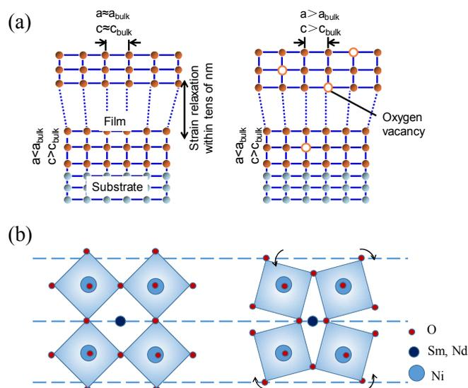
Figure 5 (a) Schematic diagram of oxygen vacancies effect on the lattice parameters in a compressively strained thin film. (b) Out-of-plane lattice parameter decrease with the Ni-O-Ni bond angle reduction.
