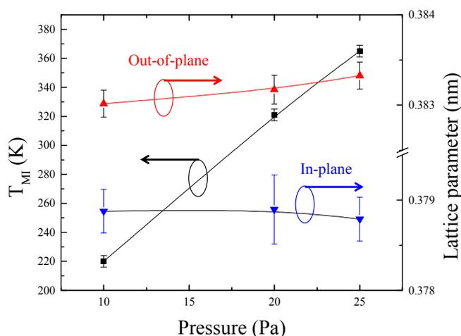
Figure 4 Film  $T_{MI}$  and lattice parameters as a function of the growth oxygen pressure.
