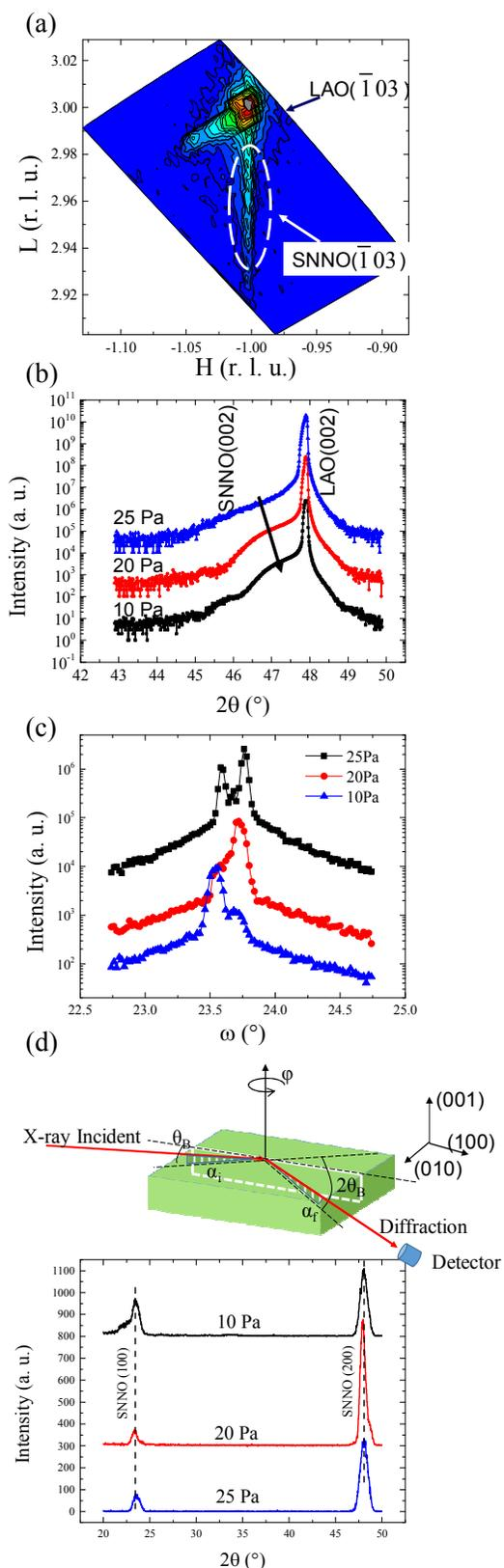
Figure 3 (a) Reciprocal space map around  $(\bar{1}03)$  reflection for the 20 Pa sample. (b) High-resolution X-ray  $\theta$ - $2\theta$  scans around the (002) reflection and (c) the corresponding rocking curves across the SNNO (002) peak. (d) Schematic illustration of in-plane GIXRD geometry and GIXRD results for a series of SNNO films.
