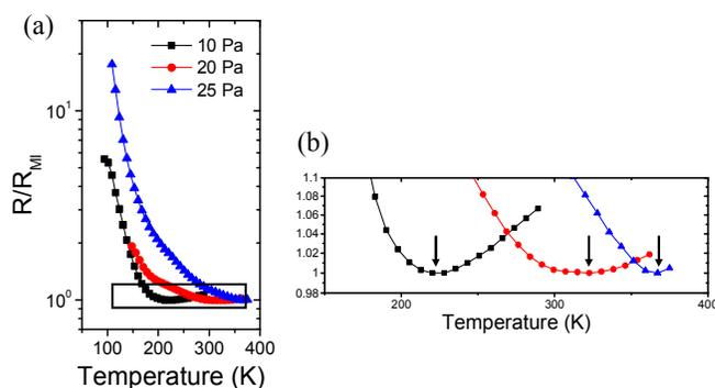
Figure 2 (a) SNNO films resistance as the function of temperature with different growth oxygen pressure. The resistance is normalized to its minimum value reached at  $T_{MI}$ . (b) The larger version of the area outlined in black in (a). The arrows indicate the  $T_{MI}$ .
