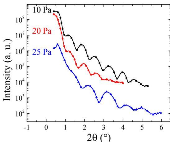
Figure 1 XRR analysis of films deposited under 10 Pa, 20 Pa, and 25 Pa, respectively.
