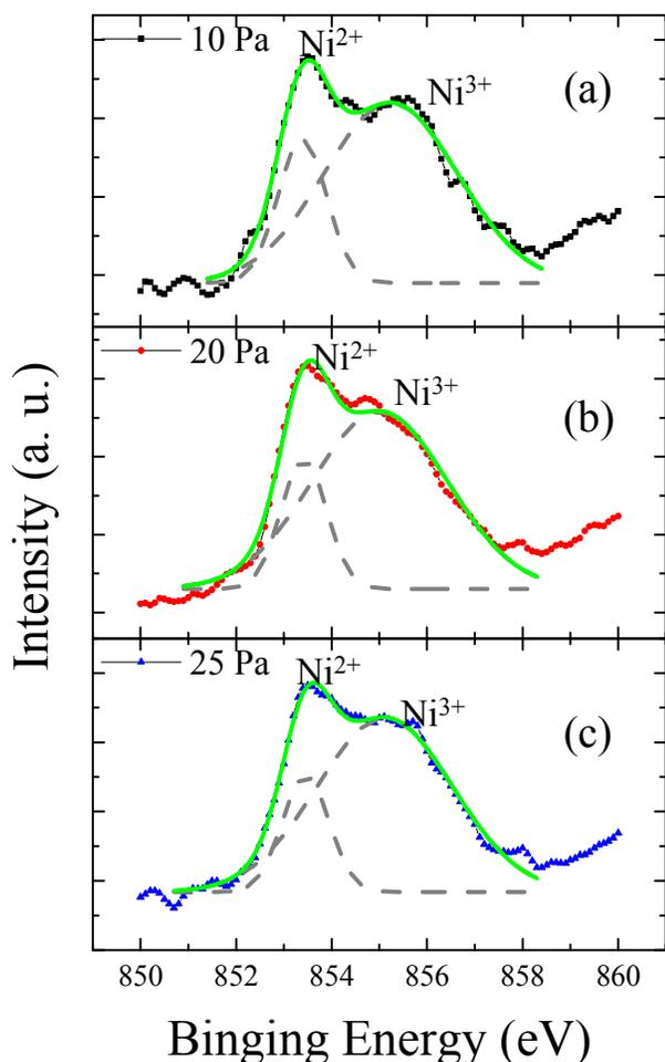
Figure 6 Ni  $2p_{3/2}$  XPS spectra of (a) 10 Pa, (b) 20 Pa and (c) 25 Pa SNNO/LAO films. The peaks associated with  $Ni^{2+}$  and  $Ni^{3+}$  are indicated.
