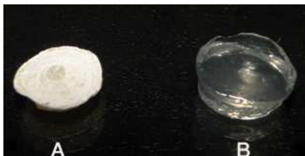
Figure 3: Synthesis of Glc-gel (above). Photograph of (A) freeze dried Glc-gel (B) swollen Glc-gel formed by radiation induced polymerization (below).
