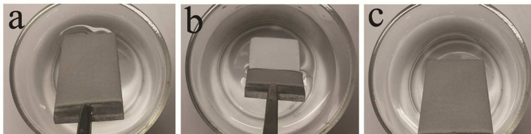
Fig. 9 (a-c) The process of the as-prepared superhydrophobic surface by immersing in and then taking out from the 3.5 wt.% NaCl solution. (Supporting Information Video 1: Air trapped test of the superhydrophobic surface by immersing in and then taking out from 3.5 wt.% NaCl solution.)
