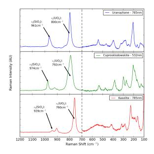
**Fig. 6** Representative Raman spectra of the uranyl silicate minerals uranophane, kasolite and cuprosklodowskite. The 100-700cm<sup>-1</sup> region has been rescaled, to emphasise the bands in this region. The wavelengths displayed correspond to the optimum excitation for each mineral. The major peaks are annotated, while all bands are listed in Tables SI 10–12.
