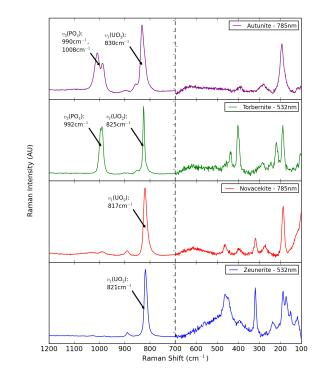
**Fig. 2** Representative Raman spectra of autunite, torbernite, nováčekite and zeunerite mineral samples. The 100-700cm<sup>-1</sup> region has been rescaled, to emphasise the bands in this region. The wavelengths displayed correspond to the optimum excitation for each mineral. The major peaks are annotated, while all bands are listed in Tables SI 1–4.
