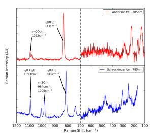
Raman spectra of the uranyl carbonate minerals
