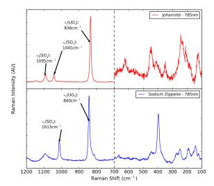
Fig. 5 Representative Raman spectra of the uranyl sulphate minerals johannite and natrozippeite. The  $100-700 \text{cm}^{-1}$  region has been rescaled, to emphasise the bands in this region. The wavelengths displayed correspond to the optimum excitation for each mineral. The major peaks are annotated, while all bands are listed in Tables SI 8 and SI 9.
