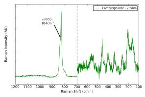
**Fig.** 7 A representative Raman spectrum of the uranyl hydrate mineral compreignacite. The 100-700cm<sup>-1</sup> region has been rescaled, to emphasise the bands in this region. The 785 nm excitation produced the best spectrum, which is shown here. The major peaks are annotated, while all bands are listed in Table SI 13.
