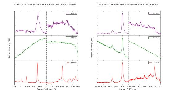
Fig. 8 A comparison of the spectra obtained using the three excitation wavelengths for the uranyl sulphate mineral natrozippeite (left) and the uranyl silicate mineral uranophane (right). The  $100-700 \text{ cm}^{-1}$  region has been rescaled, to emphasise the bands in this region.
