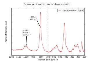
Fig. 3 A representative Raman spectrum of the mineral phosphuranylite. The 100-700 cm<sup>-1</sup> region has been rescaled, to emphasise the bands in this region. The 785 nm excitation produced the best spectrum, and is shown here. The major peaks are annotated, while all bands are listed in Table SI 5.
