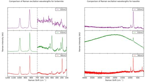
**Fig. 9** A comparison of the results obtained using the three excitation wavelengths for the uranyl phosphate mineral torbernite (left) and the uranyl silicate mineral kasolite (right). The spectrum for kasolite displays a range from 0-4000 cm<sup>-1</sup>, to show there are few peaks of interest above  $1200 \text{ cm}^{-1}$ . The  $100-700 \text{ cm}^{-1}$  region in the torbernite spectrum has been rescaled, to emphasise the bands in this region.
