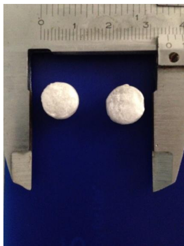
Figure 5: Paracetamol loaded silica aerogels encapsulated with alginate aerogel layers. (Hybrid aerogel at the right was synthesized after 4 months the hybrid aerogel at the left was synthesized)
