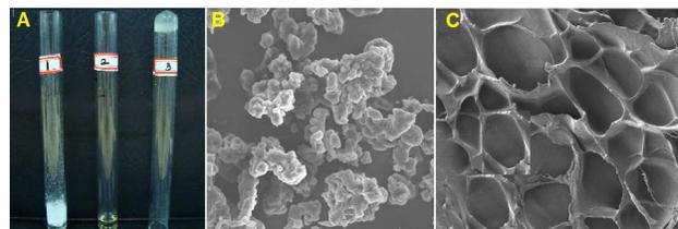
**Fig. 3** The surface morphology and photographs of the ECH-HPP hydrogel: (A) photographs of the pachyman in water (tube #1), HPP in water (tube #2) and ECH-HPP hydrogel (tube #3); (B) SEM image of HPP and (C) SEM image of the hydrogel.
