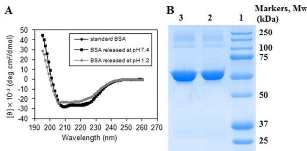
**Fig. 7** The stability test of the released BSA: (A) CD spectra of the standard BSA, BSA released at pH 1.2 and BSA released at pH 7.4 (at pH 1.2 for 2 h and then at pH 7.4 for 8 h) and (B) Coomassie-stained SDS-PAGE gel of the released BSA at pH 7.4. Lanes 1, 2 and 3 are, respectively, the molecular weight markers, BSA standard, BSA released from the ECH-HPP hydrogel at pH 7.4.
