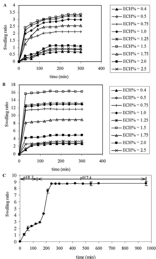
**Fig. 2** Swelling profiles of the ECH-HPP hydrogel: (A) One-step swelling characteristics of the hydrogel with different amounts of ECH at pH 1.2; (B) One-step swelling characteristics of the hydrogel with different amounts of ECH at pH 7.4 and (C) Two-step swelling characteristics of the hydrogel at pH 1.2 for 2h and subsequently in pH 7.4 for 14h.
