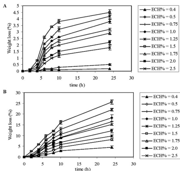
**Fig. 5** Weight loss of the ECH-HPP hydrogel as a function of immersion time in PBS (pH=7.4) at 37°C: (A) Chemical hydrolysis and (B) Enzymatic hydrolysis.
