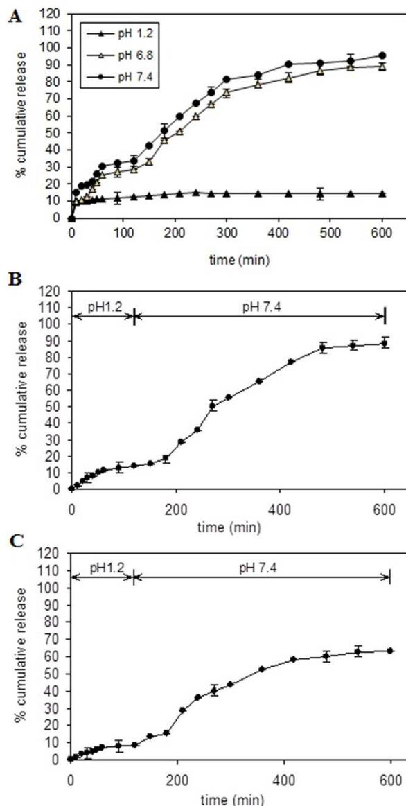
**Fig. 6** Drug release profile of the ECH-HPP hydrogel: (A) One-step BSA release profile of the hydrogel in pH 1.2 or pH 6.8 or pH 7.4, respectively; (B) Two-step BSA release profile of the hydrogel in pH 1.2 for 2h and subsequently in pH 7.4 for 8 h and (C) Two-step lysozyme release profile of the hydrogel in pH 1.2 for 2h and subsequently in pH 7.4 for 8 h.
