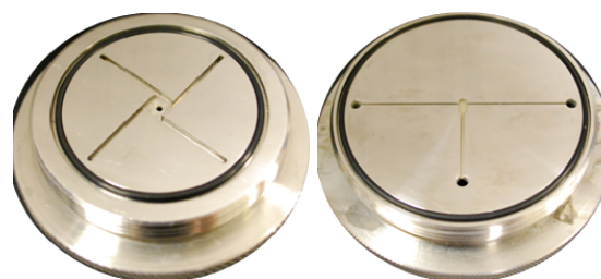
Fig. 2 Design of multi-inlet vortex mixer (MIVM) (left) and confined impinging-jet mixer (CIJM) (right).
