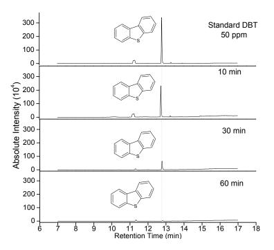
**Figure 5:** Oxidation of DBT as a function of time followed by quantitative GC-MS. Reaction conditions: [DBT] =  $50 \text{ mgL}^{-1}$ ; [H<sub>2</sub>O<sub>2</sub>/H<sub>3</sub>CCOOH] =  $3.5 \text{mmolL}^{-1}$ ; m<sub>catalyst</sub> = 10 mg; T=  $25\pm1$  °C.
