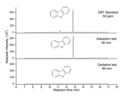
Figure 7: Comparison of DBT removal from adsorptive and oxidative tests.
