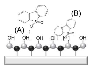
**Figure 13:** Proposal adsorption modes of DBTO<sub>2</sub> on the Red Mud surface (gray spheres are Fe, Al, Si or Ti; Black spheres are O).
