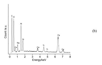
**Figure 4:** Scanning electron microscopy (SEM) coupled with energy dispersive spectroscopy (EDS) of Red Mud.
