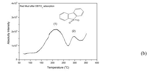
**Figure 12:** a) Adsorption of DBTO<sub>2</sub> standard after 60 min. Experimental condition: [DBTO<sub>2</sub>] = 50 mg L<sup>-1</sup>; m  $_{adsorbent}$  = 10 mg; T=25±1 °C. b) Release profile of dibenzothiophene sulfone monitored by GC-MS.
