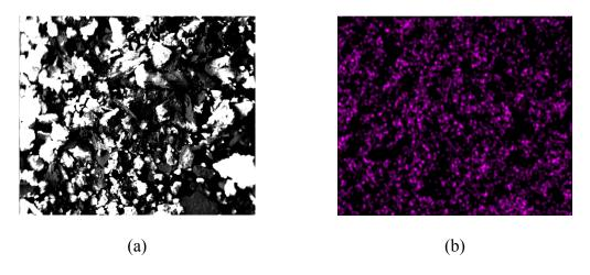
**Figure 8:** (a) SEM image and (b) EDS mapping of sulfur on Red Mud after use as a catalyst and adsorbent.
