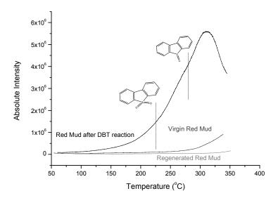
**Figure 9:** Release profile of volatile compounds monitored by GC-MS.
