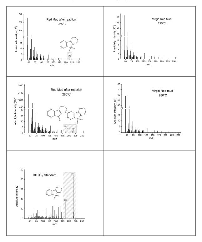
**Figure 10:** Mass spectra of ions volatilized from Red Mud after catalytic DBT oxidation and virgin Red Mud obtained at 225 °C and 280 °C.
