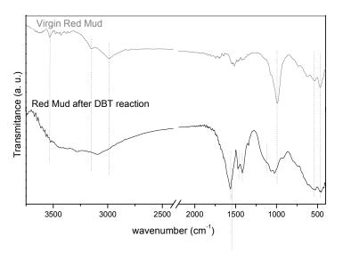
Figure 11: Infrared spectra of Virgin Red Mud and Red Mud after use as a catalyst.
