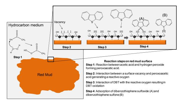
**Figure 14:** Possible mechanism of an oxidative adsorptive process of DBT on the surface of Red Mud (Gray spheres are Fe, Al, Si or Ti; Black spheres are O).
