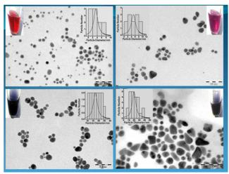
Fig.4. TEM images of AuNPs made at constant cyclohexanone (4.8M) and varying 3-APTMS concentrations of 8mM (red), 10mM (purple), 50 12mM (blue), and 15mM (violet).
