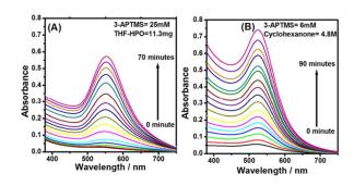
60 Fig.1 Real time synthesis of AuNPs mediated by 3-APTMS - THF-HPO (A) and 3-APTMS-cyclohexanone (B)
