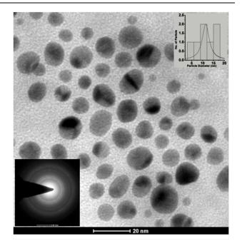
**Fig.8**.TEM image of PBNP-AuNPs nanocomposite along with respective 40 diffraction pattern.
