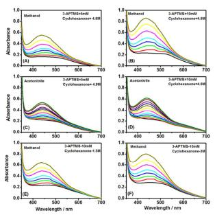
Fig.7. UV-VIS spectra of o-dianisidine-H<sub>2</sub>O<sub>2</sub> system catalyzed by AuNPs in methanol (A, B) acetonitrile (C, D) justifying the role of functional ability; Curves E and F shows results on same line as a function of <sup>5</sup> nanogeometry.
