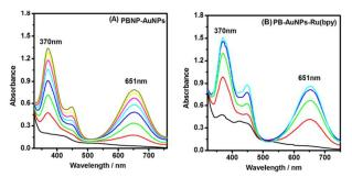
Fig.10. VIS spectra of 3, 3', 5, 5'-Tetramethylbenzidine (TMB)  $-H_2O_2$  system catalyzed PBAuRu(bpy).
