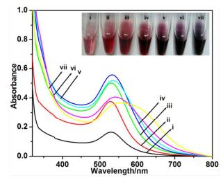
Fig.2. UV-VIS Spectra showing change in  $\lambda_{max}$  of AuNPs made using constant concentration of cyclohexanone (4.8M) and varying 65 concentration of 3-APTMS; (i) 3mM (ii)4mM (iii)6mM (iv)8mM (v)9mM (vi)10mM (vii)12mM
