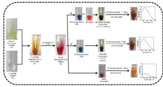
60 Scheme.2. Schematic presentation of various stages of nanocomposite formation for homogeneous catalysis.
