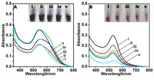
**Fig.3.** UV-VIS Spectra showing change in  $\lambda_{max}$  of AuNPs made using : 5 (A) constant concentration of 3-APTMS (10mM) and varying cyclohexanone concentration (i)1.0 M, (ii)1.5M, (iii) 2.0M, (iv) 3.0M (v)4.0M; (B) constant concentration of 3-APTMS (5mM) and varying cyclohexanone concentration; (i) 4M (ii) 5.0M (iii) 6.0M (iv) 7.0M (V) 8.0M
