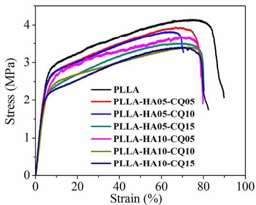
**Figure 6.** Stress-strain curves of electrospun fibrous membranes, respectively.
