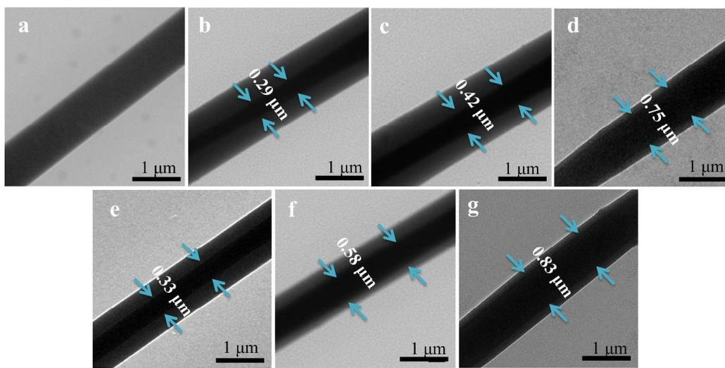
**Figure 3.** TEM images of core-shell structures of PLLA (a), PLLA-HA05-CQ05 (b), PLLA-HA05-CQ10 (c), PLLA-HA05-CQ15 (d), PLLA-HA10-CQ05 (e), PLLA-HA10-CQ10 (f), and PLLA-HA10-CQ15 (g) fibers, respectively.
