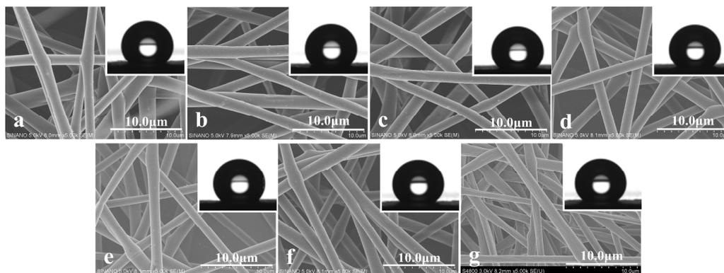
**Figure 2.** SEM images of PLLA (a), PLLA-HA05-CQ05 (b), PLLA-HA05-CQ10 (c), PLLA-HA05-CQ15 (d), PLLA-HA10-CQ05 (e), PLLA-HA10-CQ10 (f), and PLLA-HA10-CQ15 (g), respectively. The corresponding images in WCA tests are shown in the insets.
