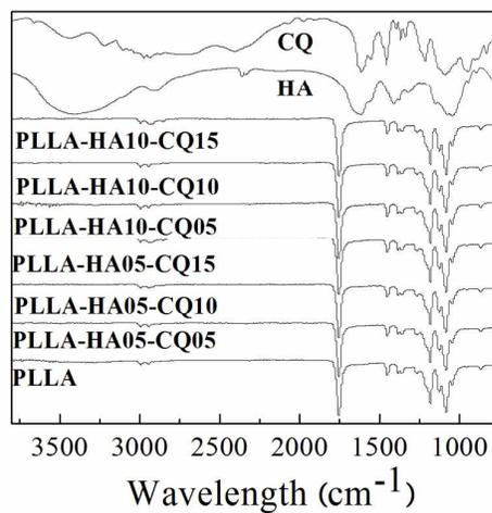
**Figure 4.** FTIR spectra of CQ and HA and various electrospun fibrous membranes.
