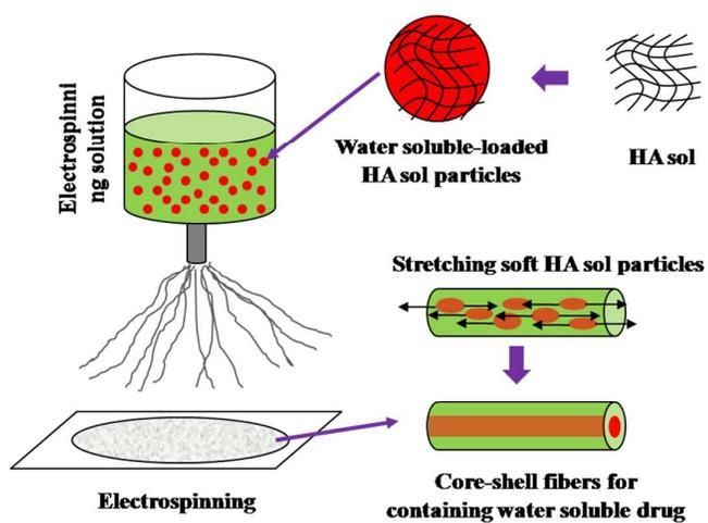
Microsol-electrospinning technique for facile fabricating core-shell microfibers to achieve incubated, controlled and sustainable release of water-soluble drugs.
