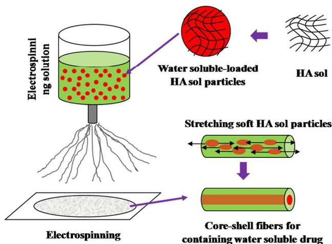
**Figure 8.** Schematic illustration of the formation of composite fibers with core-shell structure during microsol-electrospinning.
