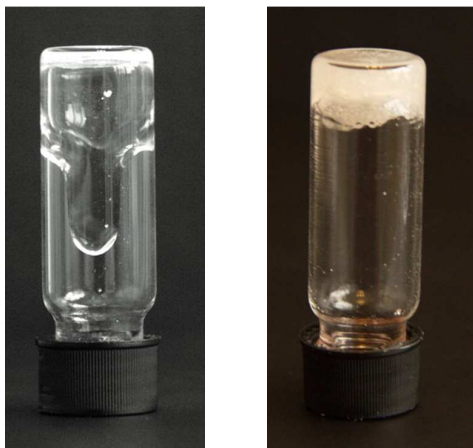
Figure 5a (left), 5b (right). Photograph of mixtures containing the PMMA/HMS-301 microcapsule and V35 after curing at 50°C (left) and 120°C (right).
