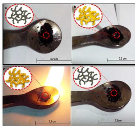
**Fig.3:** (a) Crude CS before absorption. (b) Absorption of oil by CS. (c) burning of wet CS. (d) burnt CS
