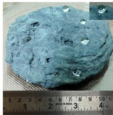
**Fig.1:** Hydrophobicity of PVDF-CS composite is demonstrated by dripping water droplets on the surface of composite.
