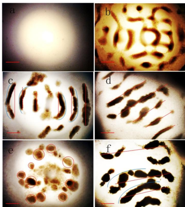
Figure 3. The assembling process of nanoparticles in the droplet with the sodium chloride concentration of 0.144 g/mL and the scale bar is 500 \mu\text{m} . (a) Particles distribute in the droplet uniformly before the SSAWs are applied. (b) Particles gather in short chains. (c) Particles assemble in lines perpendicular to the SAW wave line. The red lines indicate particles gather in lines, and blue curves indicate the curling particle chains. (d) Particles lines are moving from the direction perpendicular to SAW propagation to that having an angle with the electric field line by increasing F_{DEP} . The red lines indicate the direction of the particle chains. (e) Particle chains are broken up to form islands in the droplet with further increasing of F_{PDE} . (f) The F_{DEP} dominates the behaviors of particles concentration, and particles gather in lines along the electric field line when the distance between particles and the substrate decreases to short enough.
