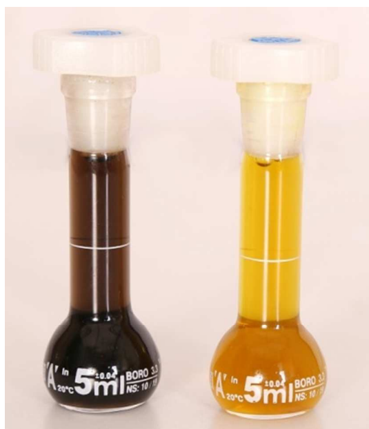
Fig. 1 Digital photograph of Pd 0.5 -Ni 0.5 B-NPs before (right-hand) and after (left-hand) reduction with hydrazine hydrate.
