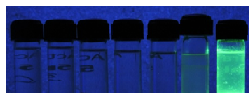
Fig.2 PL spectra of 2 and 3 in DCM/hexane mixed solvents with different f_H with excitation at 385 nm [for (i) and (iv) for 2 and 3 , respectively], ( \lambda_{\text{max}} : a=479 and b=512 nm for 1 and a=490 and b=517 nm for 2 ); Variation of PL intensity with respect to changes of wavelength with inclusion of error bar [(ii) and (v) for 2 and 3 , respectively]; Luminescent images of 2 and 3 [(iii) and (vi) for 2 and 3 , respectively] (irradiated with an ultraviolet light at 365 nm) in hexane-DCM mixed solvents with the concentration kept at 2 \times 10^{-5} \text{ mol}\cdot\text{L}^{-1}
