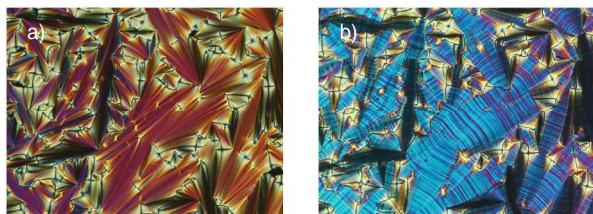
Fig. 4. The optical textures of a) SmA phase (205 °C) and b) E phase (175 °C) obtained for 1[12]c –[Pyr] c on cooling from the isotropic phase in the same region of the sample.
