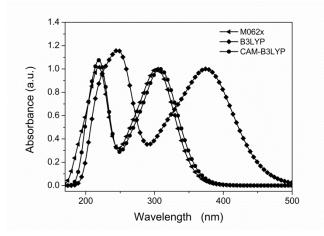
Figure 4 Computed Uv-vis absorption spectra of  $\mathsf{BOXD}\text{-}\mathsf{NP}$  with different methods.
