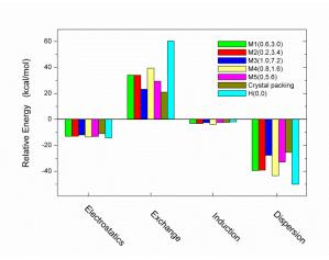
Figure 8 Intermolecular interaction energy components of BOXD-NP dimers. M1-M5 (offset  $\pi$ -stacking) are the energy-minimum molecular stacking structures of BOXD-NP found in the PES surface scanning. Crystal packing is obtained from single crystal X-ray analysis. H(0,0) refers to the ideal face-to-face  $\pi$ -stacking configuration.
