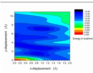
Figure 6 Contour image of intermolecular interaction potential energy surface of BOXD-NP. The potential energies were computed as a function of molecular shifts along both the molecular long axis (*y*-displacement, and *y* for short) and short axis (*x*-displacement, and *x* for short) with M062x/6-31G\*\* method based on a dimer model.
