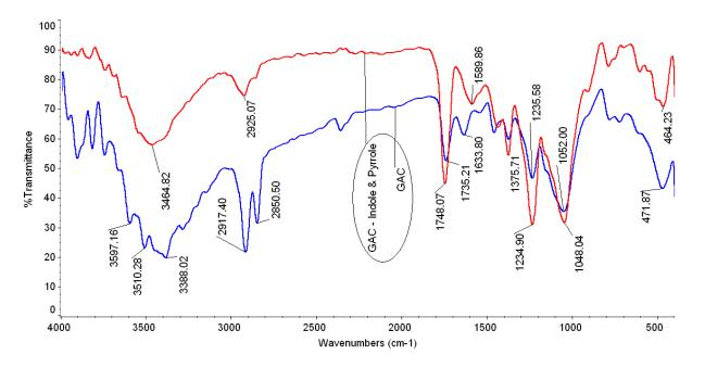
Fig. 3 FTIR of GAC before and after adsorption
