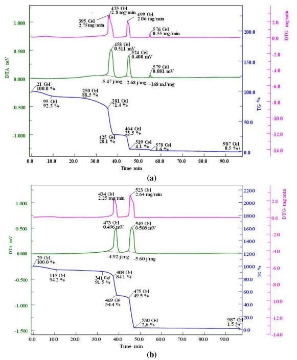
Fig. 2 Thermogravimetric analysis under air atmosphere (a) GAC blank and (b) GAC loaded with pyrrole and indole.
