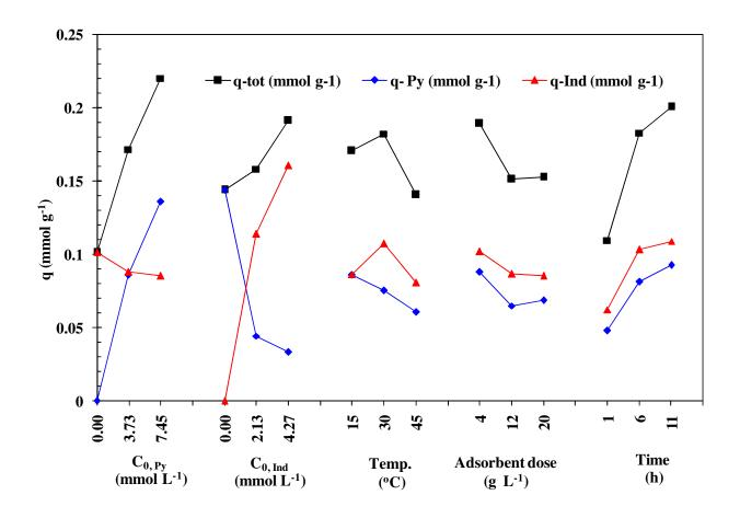
Fig. 4 Effect of process parameters on  $q_{\text{tot}}$  for multicomponent adsorption of pyrrole and indole onto GAC
