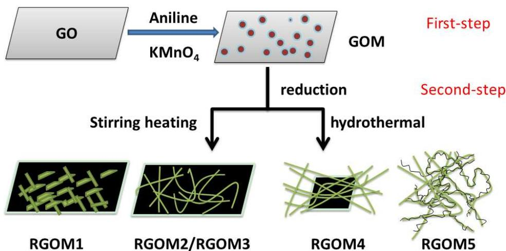
**Scheme 1** Schematic illustration of two-step synthesis of GOM and RGOM.
