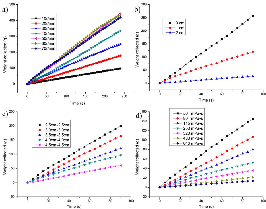
Figure 6: a) Weight collected at different revolving rates of pump. b) Oil collection rates with different distances of oil surface to pipe nozzle. c) Oil collection rates with different superficial area. d) Oil collection rates under different viscosities of oil.
