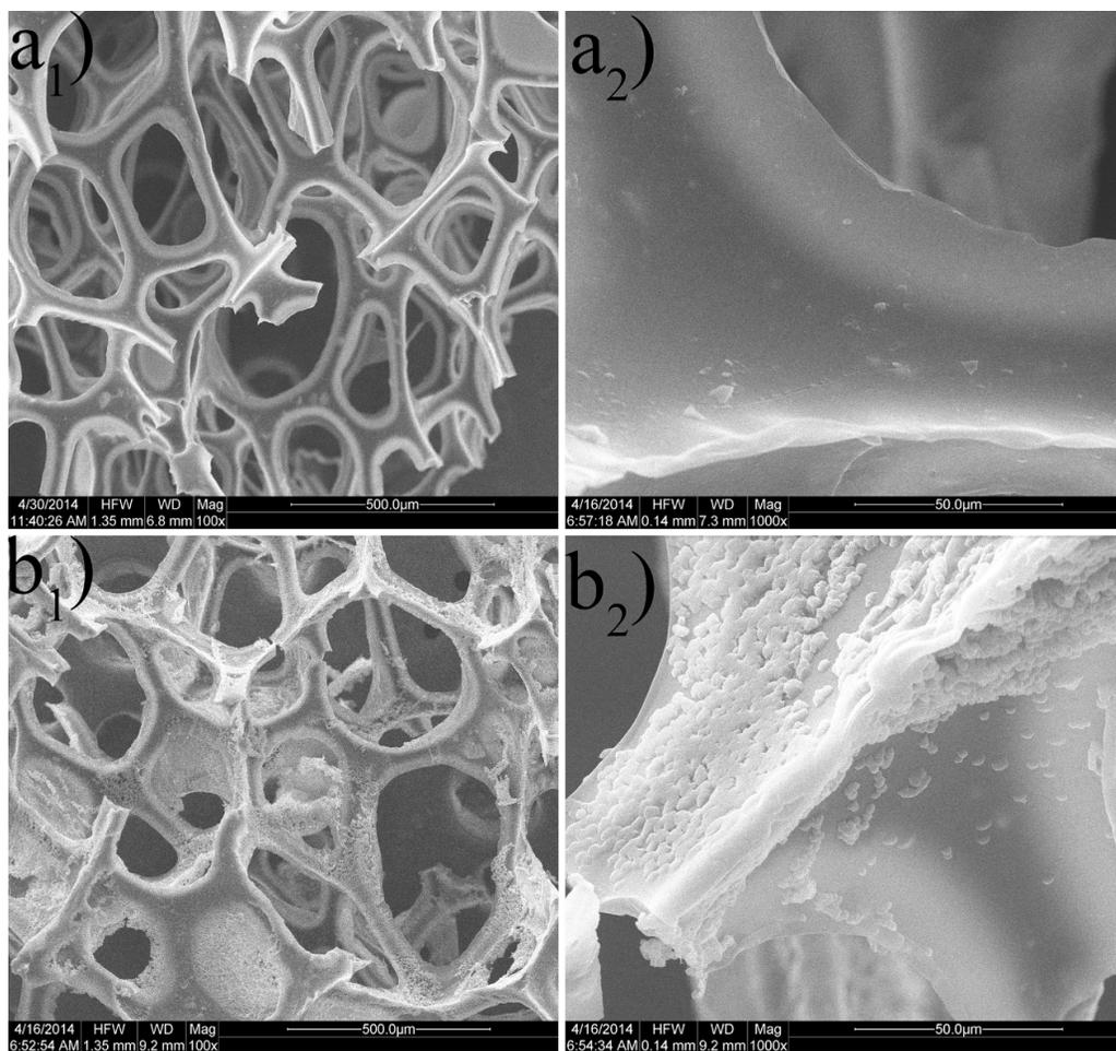
Figure 3: SEM images of PU sponges before (a<sub>1</sub>, a<sub>2</sub>) and after (b<sub>1</sub>, b<sub>2</sub>) modification at different magnifications
