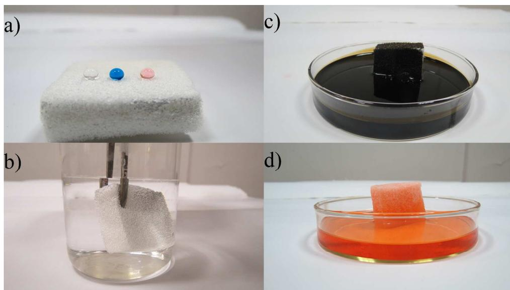
Figure 2: a) Three kinds of water droplets (pH=1, 7, 14) stand on the sponge surface with spherical shapes. b) The modified sponge is pressed into water with small air bubbles attaching around the surface. c) The modified sponge is saturated with crude oil quickly. d) The modified sponge is saturated with organic solvent (n-hexane as an example) quickly.
