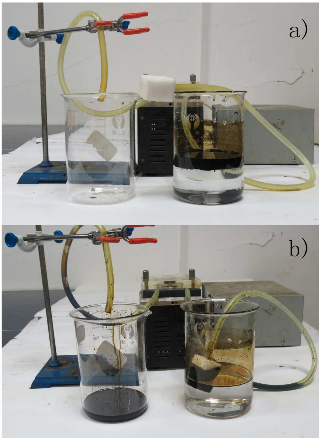
Figure 5: Separation of water and oil by pump.
