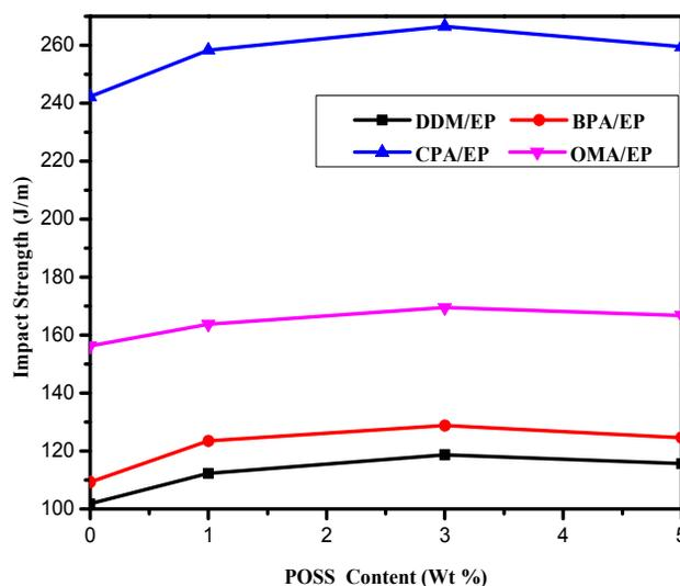
**Figure 4 Effect of POSS reinforcement on impact strength of diamine cured epoxy composites**
