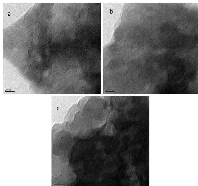
**Figure 7 TEM micrograph of 1%, 3% and 5% POSS reinforced CPA diamines cured epoxy matrix**
