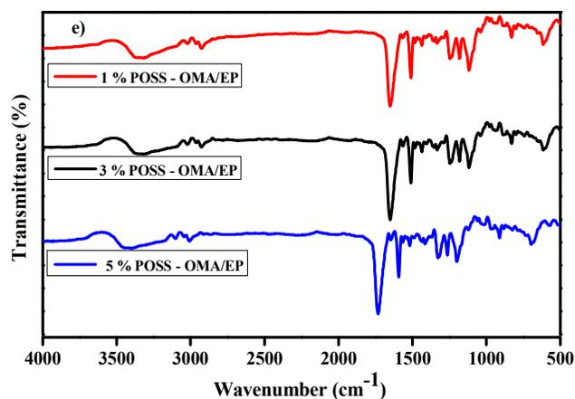
**Figure 1 FT – IR Spectra of epoxy POSS composites**
