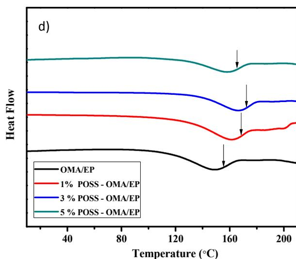
**Figure 2 DSC profile of epoxy matrix and POSS composites**
