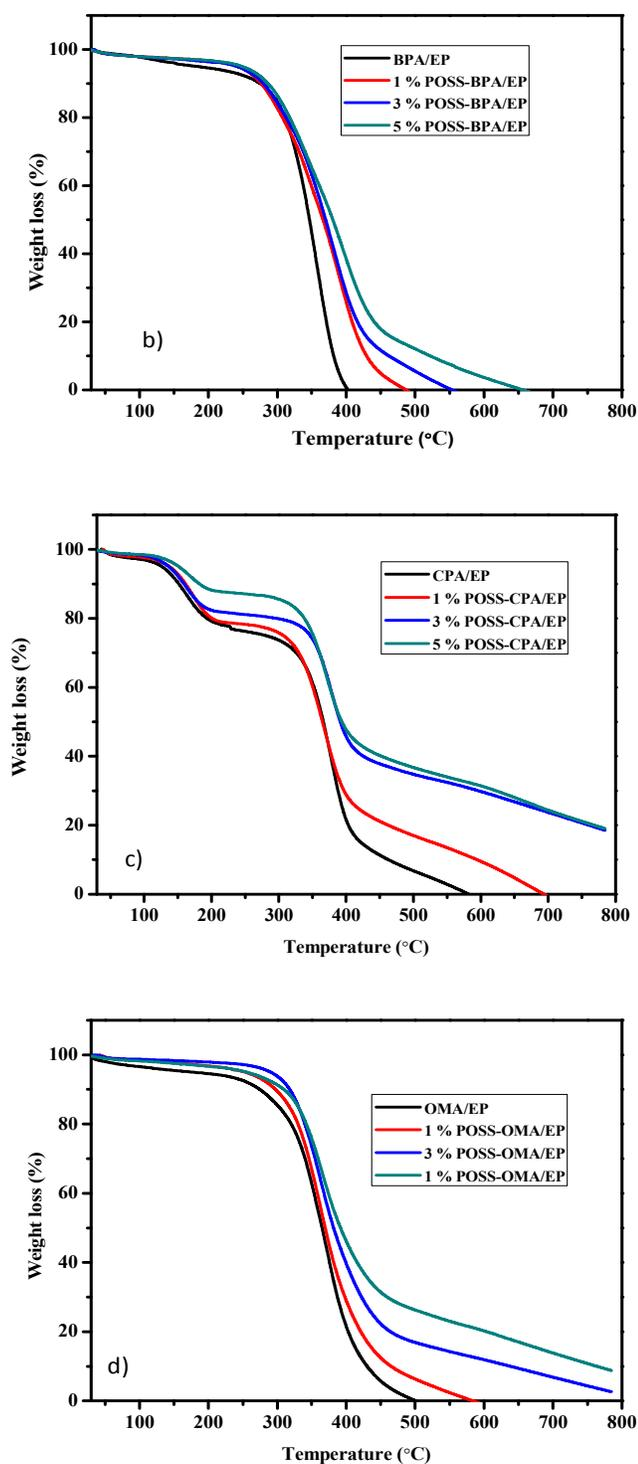
**Figure 3 TGA profiles of epoxy matrix and POSS composites**
