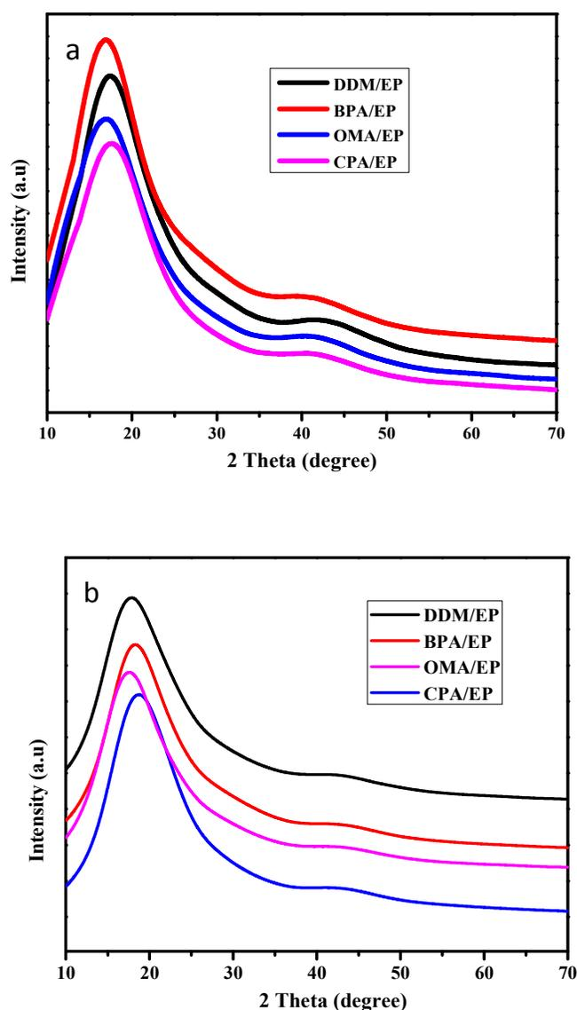
**Figure 5 XRD diffractogram of (a) Diamine cured epoxy matrices and (b) 3wt% POSS reinforced diamine cured epoxy composites**
