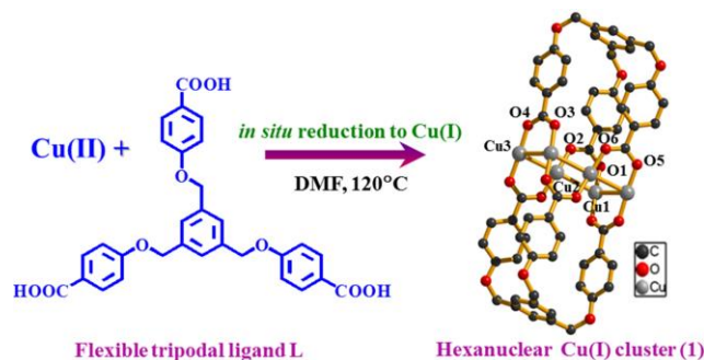
Fig. 1 Synthesis and structure of a hexanuclear complex \{Cu_3(L)_2\}_2 ( 1 ) using a novel tripodal carboxylate linker.
