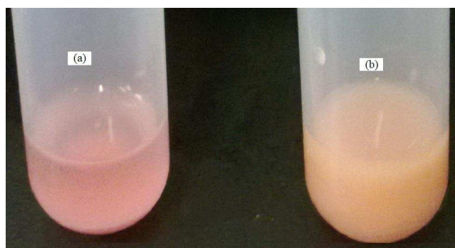
Figure 4. Images of poly(MAA-co-EGDMA) microspheres (a) and hairy particles (1) (b) in DMF/H 2 O (95/5) at 0°C for 2 h.
