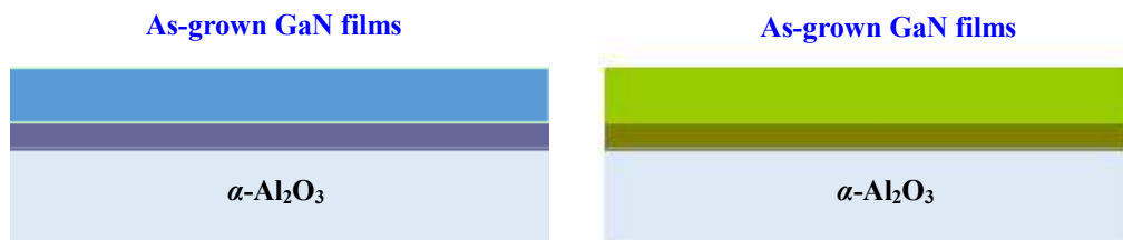
Fig. 8. Schematic diagrams for the GaN films grown on (a) nitrided, and (b) non-nitrided \alpha -Al 2 O 3 substrates, respectively.
