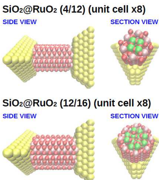
Figure 3. Side and section views of fragments of the SiO 2 @RuO 2 (4/12) and (12/16) nanowires between gold electrodes with the shape of a truncated pyramid. The length of the nanowire fragments is eight times the unit cell. O, Si, Ru and Au atoms are represented by red, green, pink and yellow spheres, respectively.
