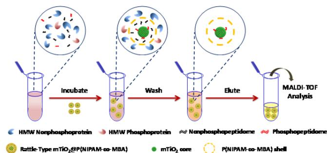
**Scheme 2** Schematic illustration of the typical process for selective extraction of phosphopeptide by using rattle-type mTiO<sub>2</sub>@P(NIPAM-co-MBA) microspheres.
