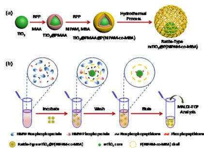
Rattle-type  $m\text{TiO}_2@P(\text{NIPAM-co-MBA})$  microspheres with a screening gel network shell were elaborately designed and fabricated for highly extraction of endogenous phosphopeptide.
