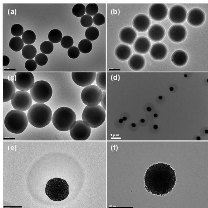
**Fig. 1** Representative TEM images of (a)  $\text{TiO}_2$ , (b)  $\text{TiO}_2$ @PMAA, (c)  $\text{TiO}_2$ @PMAA@P(NIPAM-co-MBA), (d, e) rattle-type  $\text{mTiO}_2$ @P(NIPAM-co-MBA) and (f)  $\text{mTiO}_2$ . (The scale bars are 300 nm for a, b, c, e, f and 1  $\mu\text{m}$  for d)
