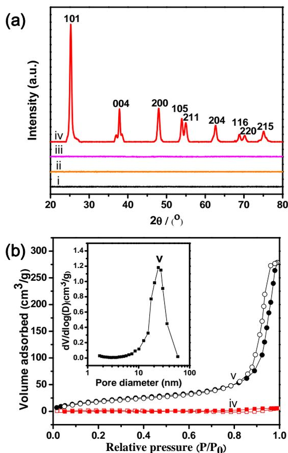
**Fig. 3** (a) X-Ray diffraction patterns of (i) TiO<sub>2</sub>, (ii) TiO<sub>2</sub>@PMAA, (iii) TiO<sub>2</sub>@PMAA@P(NIPAM-co-MBA) and (iv) rattle-type mTiO<sub>2</sub>@P(NIPAM-co-MBA); (b) nitrogen adsorption–desorption isotherms (●=adsorption, ○=desorption) curves of (iv) rattle-type mTiO<sub>2</sub>@P(NIPAM-co-MBA) and (v) mTiO<sub>2</sub> (the inset is the BJH pore-size distribution of mTiO<sub>2</sub>).
