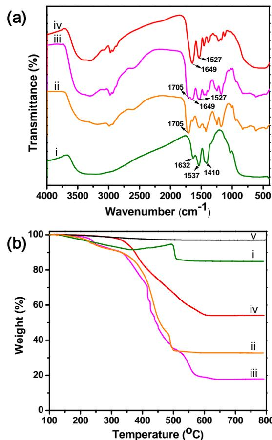
**Fig. 2** (a) FT-IR spectra and (b) TGA curves of (i)  $\text{TiO}_2$ , (ii)  $\text{TiO}_2$ @PMAA, (iii)  $\text{TiO}_2$ @PMAA@P(NIPAM-co-MBA), (iv) rattle-type  $\text{mTiO}_2$ @P(NIPAM-co-MBA) and (v)  $\text{mTiO}_2$ .
