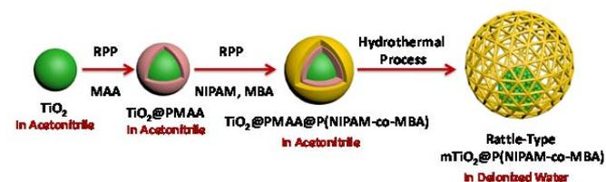
**Scheme 1** Schematic illustration of the synthetic procedure for preparation of rattle-type  $\text{mTiO}_2@\text{P}(\text{NIPAM-co-MBA})$  microspheres.
