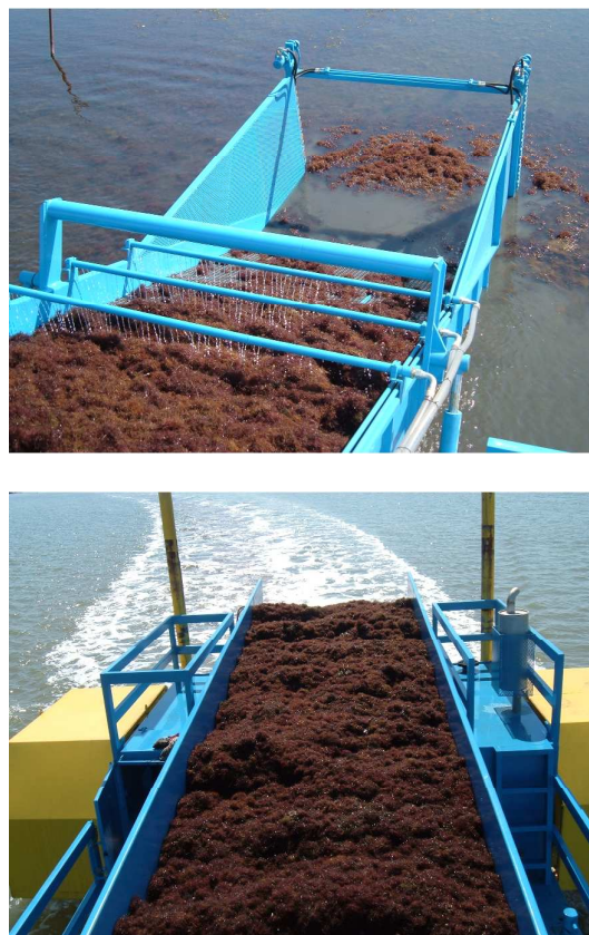
Figure 1. Mechanical harvesting process of Gracilaria gracilis in the Lesina lagoon (Italy).
