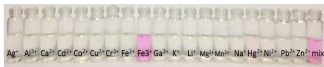
Fig 1. Changes in the visible light of P1 (50 μM) in ethanol-Tris-HCl buffer (v/v, 1/9, pH = 7.0) solutions upon addition of various metal ions (10equiv.). Mix means P1 with all kinds of metal ions.
