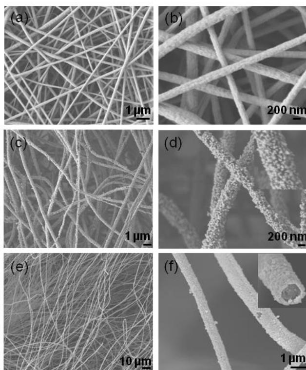
**Figure 2.** SEM images (a) and (b) of the electrospun polymer nanofibers, (c) and (d) of the polymer nanofibers coated with silver nanoparticles and (e) and (f) uniform silver nanoparticle coating using wetting solution.
