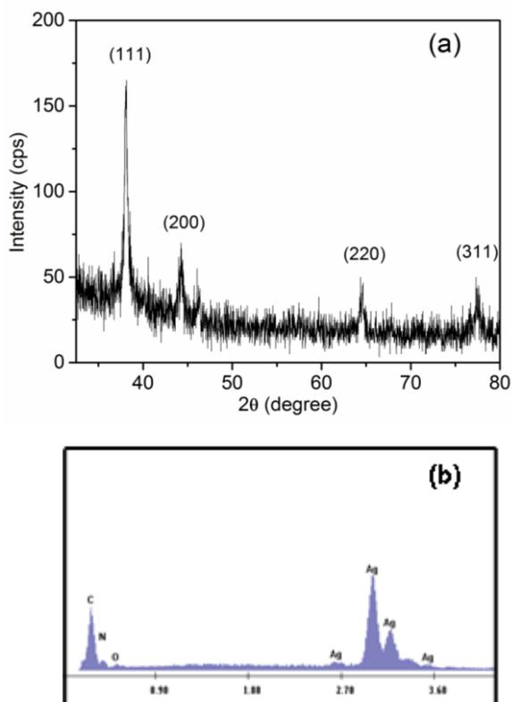
**Figure 4.** (a) XRD pattern and (b) EDS of the silver NTs.
