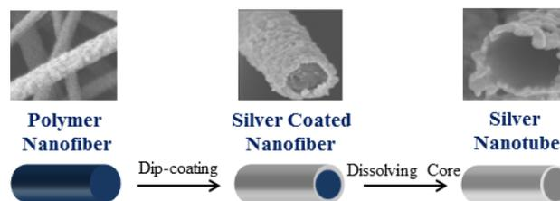
**Figure 1.** Schematic of the steps involved in the fabrication of silver NTs: Fabricating polymer nanofibers by electrospinning, dip coating silver nanoparticles on the nanofibers and forming silver NTs by washing away the polymeric fiber core.
