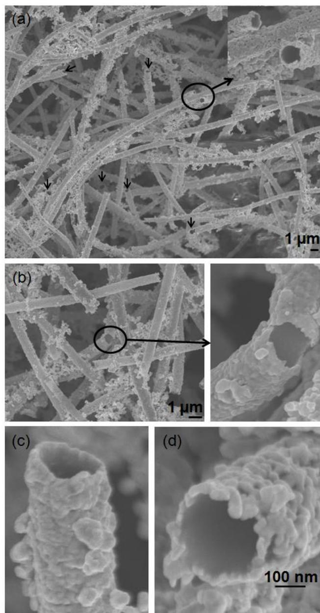
**Figure 3.** SEM images (a) of synthesized silver NTs, (b) of a broken NT at two different magnifications and (c) and (d) views of two silver NTs at high magnification.
