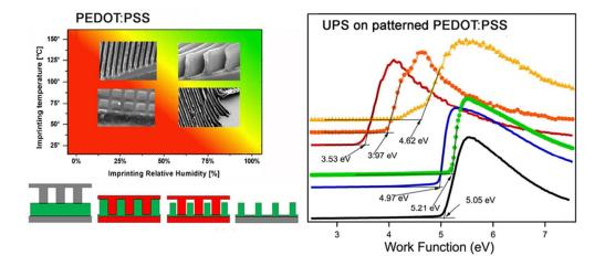
A modified Nanoimprinting Lithography process performed at high relative humidity was developed for highresolution pattering of the conductive polymer PEDOT:PSS. The process induce important effect on the electronic properties of the material, including enhanced conductivity and strong shifts in the work function and valence band edge. 36x16mm (600 x 600 DPI)
