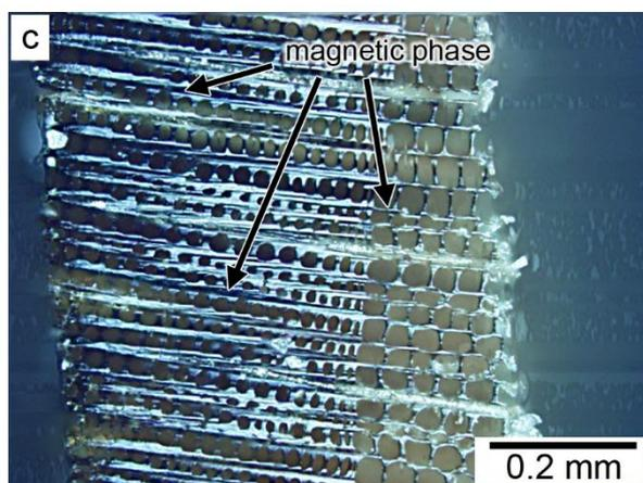
Figure 2. Optical microscopy pictures of cross-sections of a modified wood veneer specimen. a.) unmodified wood veneer (v-U); b.) wood veneer modified with ca. 8 wt.% Fe<sub>3</sub>O<sub>4</sub> (v- Fe<sub>3</sub>O<sub>4</sub>); and c.) wood veneer modified with ca. 20 wt.% Fe<sub>3</sub>O<sub>4</sub> (v-Fe<sub>3</sub>O<sub>4</sub>).
