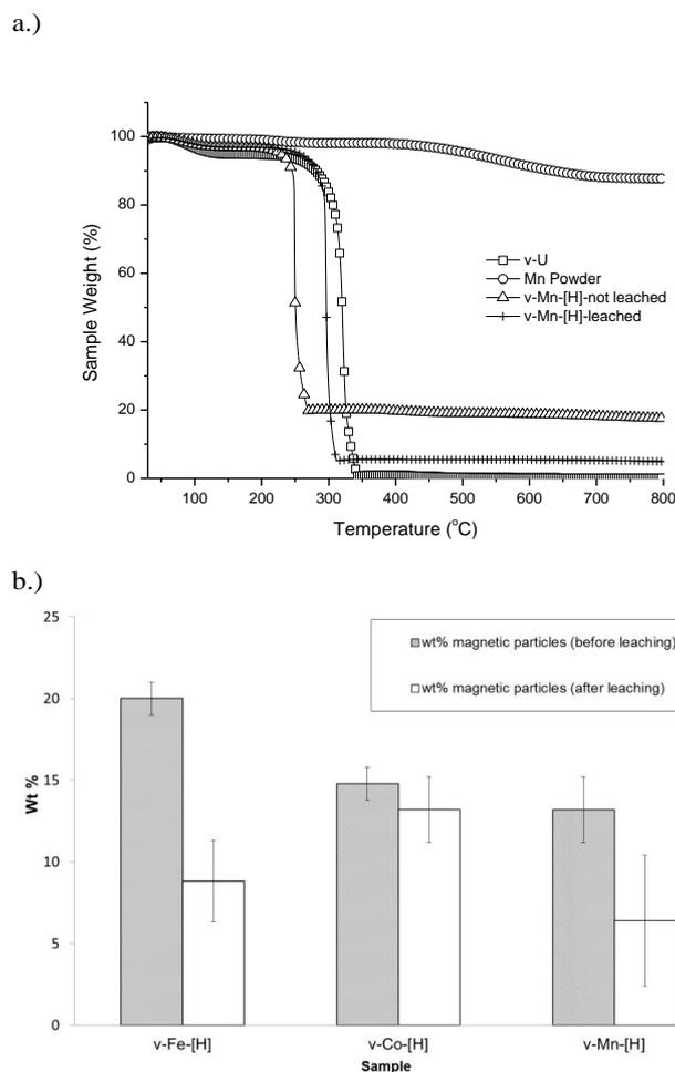
**Figure 6.** a.) TGA plot of samples and the observance of remaining magnetic particles at 750 °C b.) Summary of Weight Percent Gain (WPG) and leaching of the unmodified and modified wood veneer specimen.
