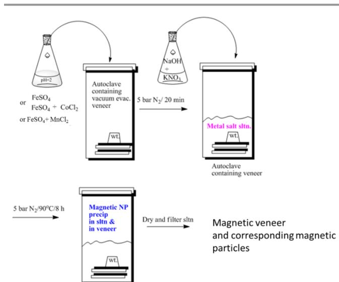
Figure 1. Overview of the process for fabrication of magnetic particle modified wood veneers.
