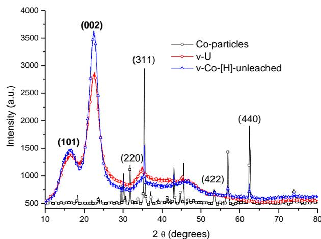
Figure 8. WAXD spectra of  $\text{CoFe}_2\text{O}_3$  samples with crystal planes from wood in bold.
