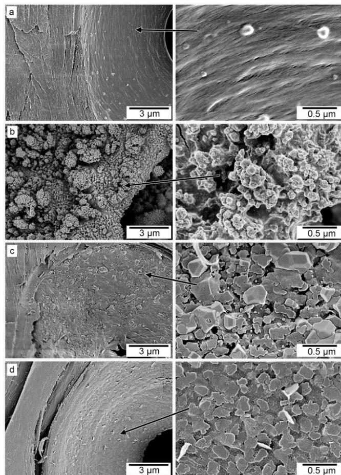
**Figure 4.** Morphology of a particles on a pore connecting wood tracheids. in a.) untreated, b.)  $v\text{-Fe}_3\text{O}_4$  c.)  $v\text{-CoFe}_2\text{O}_4$ , and d.)  $v\text{-MnFe}_2\text{O}_4$
