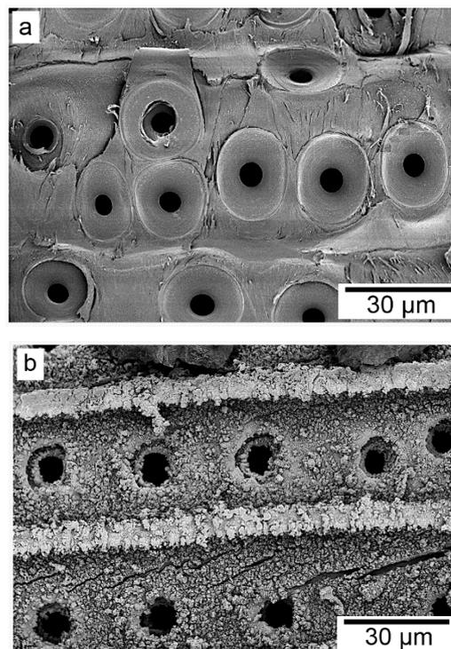
Figure 3. Lumen walls of the wood containing pores a.) v-U and b.) v- Fe<sub>3</sub>O<sub>4</sub>.
