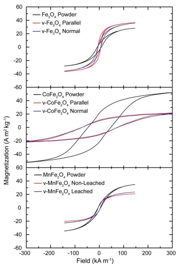
Figure 7. Magnetic hysteresis measurements of modified veneers and powder compacts demonstrating the big difference in magnetic properties between soft and hard magnetic materials. It also shows the effects of fibre orientation and leaching: a) iron ferrite  $\text{Fe}_3\text{O}_4$ , b) manganese ferrite  $\text{MnFe}_2\text{O}_4$ , c) cobalt ferrite  $\text{CoFe}_2\text{O}_3$ . Magnetisation values are normalised with respect to amount of magnetic material.
