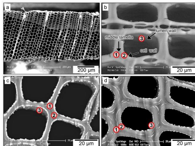
**Figure 5.** SEM micrographs of the cross section of untreated wood (a and b), and  $v\text{-Fe}_3\text{O}_4$  modified c) early wood, d) late wood.
