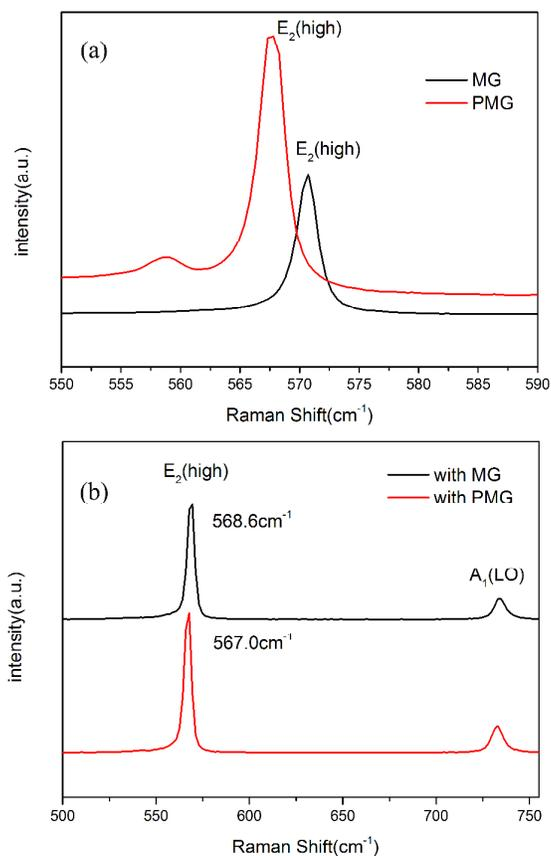
Fig.4 Raman spectra of (a) the MG and PMG substrate and (b) GaN crystals grown on the MG and PMG by HVPE
