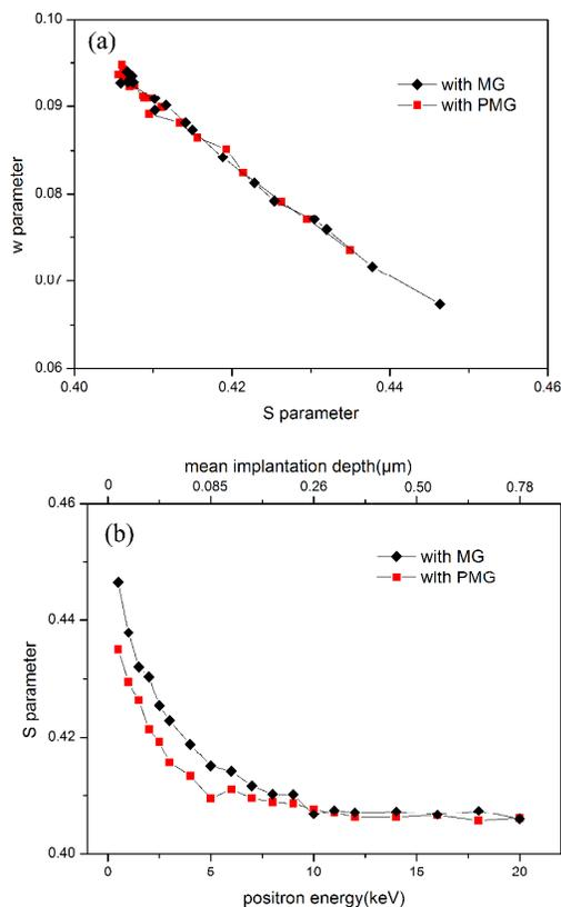
**Fig. 6** (a) Electron-momentum parameters S and W in the GaN crystals grown on MG and PMG (b) S parameter measured as a function of the positron incident energy for GaN crystals grown on MG and PMG
