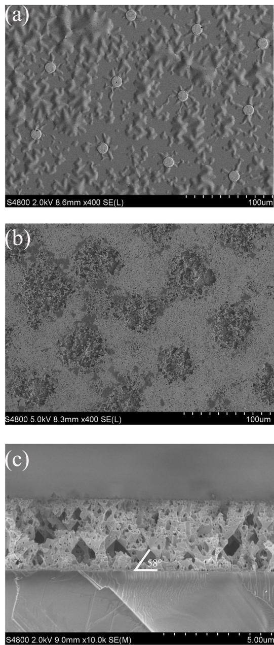
**Fig. 1** SEM images of the porous substrate (a) top view of the sample after being annealed (b-d) surface of the sample after ultrasonic process (e-f) sectional view of the porous sample after being cleaned
