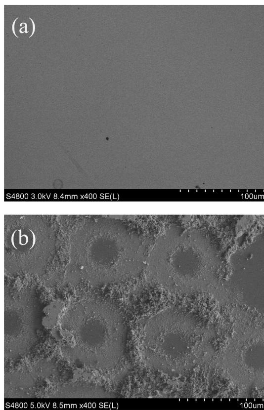
**Fig.2** SEM images of samples (a) with a complete  $\text{SiO}_2$  and (b) with the patterned masks after being annealed for 4h
