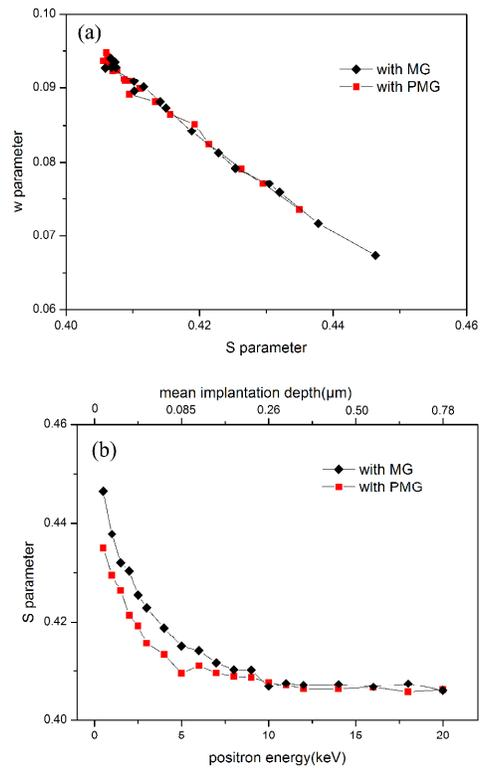
**Fig. 6** (a) Electron-momentum parameters S and W in the GaN crystals grown on MG and PMG (b) S parameter measured as a function of the positron incident energy for GaN crystals grown on MG and PMG
