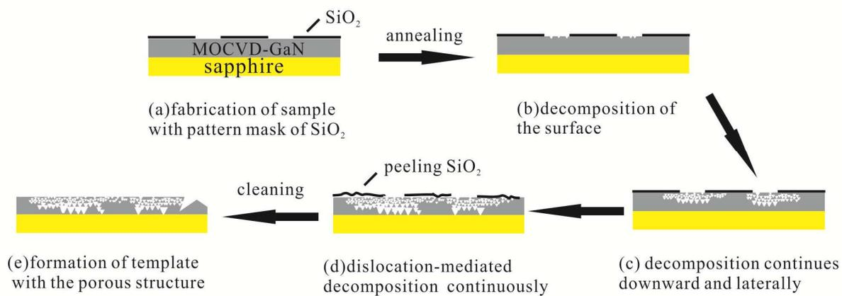
**Fig. 3** Schematic of the porous substrate formation by the HTA process
