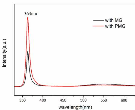
Fig. 5 PL spectra of GaN crystals grown on MG and PMG
