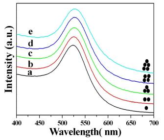
**Fig.** 7 UV-vis absorption spectra of (a) Au NPs solution and (b) two-, (c) three-, (d) four- and (e) five-AuNPs NAs solutions prepared by the dsDNA self-assembly strategy.
