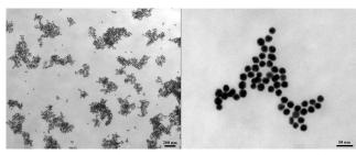
**Fig. 3** (A) TEM of the large Au NAs prepared by stepwise assembly. The Au NPs were first coupled with DNA1 and cDNA1 individually (molar <sup>55</sup> ratio: 1:60), and the resulting DNA1-Au NPs and cDNA1-Au NPs were then mixed to directly give the large Au NAs without gel electrophoresis separation; (B) TEM image of a representative large Au NA.
