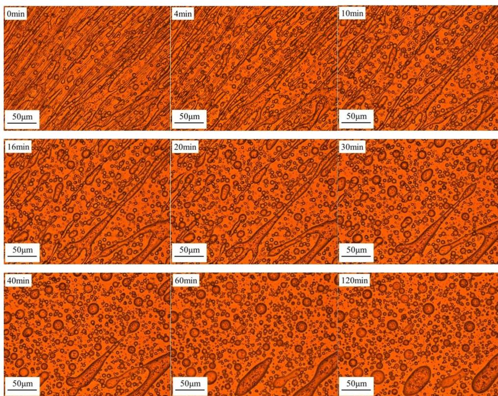
**Figure 3 Morphology development of pure PP/PS 70/30 blend observed via an optical microscope in real time during annealing at 190°C**
