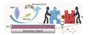
The PEI/P(DMA-*co*-PEGMEMA) multiple bilayers-coated surfaces can effectively reduce microfouling and macrofouling.
