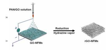
Fig. 2 Schematic illustration for fabrication of rGO-NFMs. The schematic includes of the fabrication of GO-NFMs by 40 electrospinning technique and the formation of rGO-NFMs after reduction hydrazine vapor treatment.
