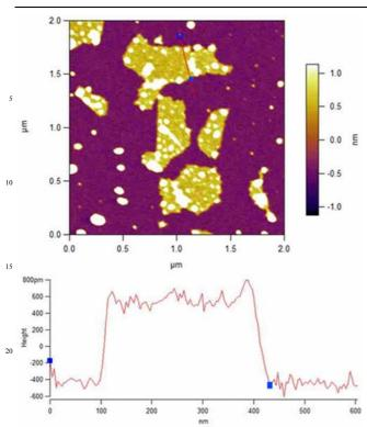
25 Fig. 1 AFM image and thickness of measured GO sheets.
