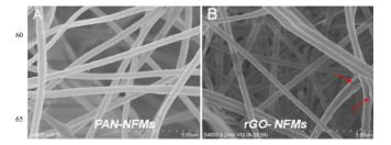
Fig. 3 SEM images of PAN-NFMs (A) and rGO-NFMs (B). The location denoted by red arrow is rGO sheets out of nanofibers.
