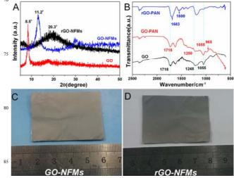
Fig. 4 XRD (A), FTIR (B) spectra of GO, GO-NFMs and rGO-NFMs. And optical photographs of (C) GO-NFMs, (D) rGO-90 NFMs.
