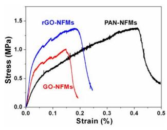
**Figure 5.** Mechanical tensile stress and tensile strain of NFMs, GO-NFMs and rGO-NFMs, respectively.
