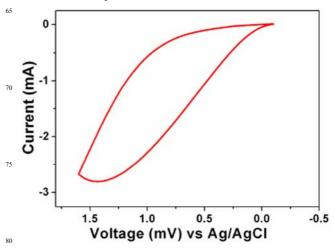
**Fig. 7** Cyclic voltammetry of the rGO-NFMs.
