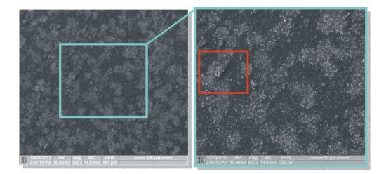
Fig. 1. Example of SEM images of nanoparticles distribution in PEM – smaller frame indicates area used for FIB thin foil preparation.
