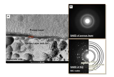
Fig. 2. Cross section TEM analysis of the silicon carbide nanoparticles introduction into porous polymer coatings: a) bright field image; b) selected area electron diffraction patterns. The red arrow indicates a border between polymer porous layers. 310x177mm (96 x 96 DPI)
