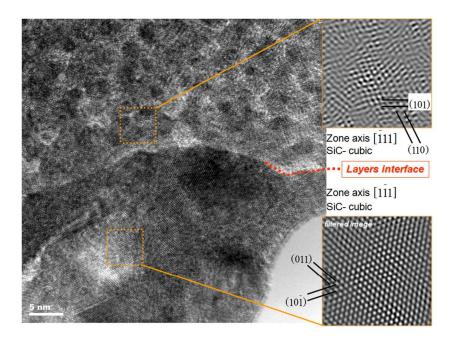
Fig. 3. HRTEM analysis of the silicon carbide nanoparticles introduction into porous polymer coatings. 310x191mm (96 x 96 DPI)
