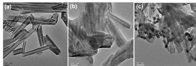
**Fig. 3** TEM images of HNTs (a) modified HNTs with P4VP (b) and HNTs loaded with Cu NPs (c)
