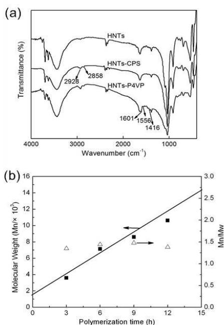
**Fig. 2** FTIR spectra of HNTs, HNTs-CPS and HNTs-P4VP (a) and Evolution of Mn and Mw/Mn vs polymerization time (b)
