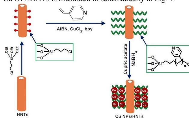
**Fig. 1** Schematic illustration of the overall preparation process of Cu NPs/HNTs
