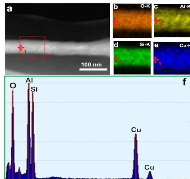
**Fig. 4** Element mapping of Cu NPs/HNTs via EDX: image (a) is the sample; images (b, c, d, and e) exhibit the element sensitive maps of oxygen, aluminum, silicon, and copper. The complete element distribution is seen in the EDX spectrum in (f)
