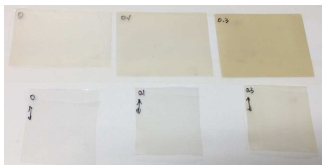
Fig. 3 Untreated and stretched films (The arrow indicates the stretching direction). The more AgNWs contained, the less transparent. Compared to untreated films, the stretched films are more transparent.
