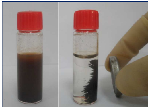
Fig. 7. Separation of the nanocatalyst from the reaction mixture by an external magnet.
