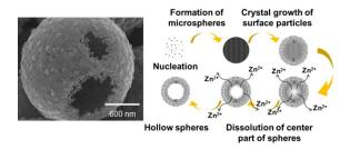
ZnO hollow microspheres exhibiting only c planes on the surface were successfully synthesized by a solvothermal method even without using template. The ZnO hollow microspheres are formed by preferential dissolution of centers of ZnO solid microspheres which have low crystallinity.
