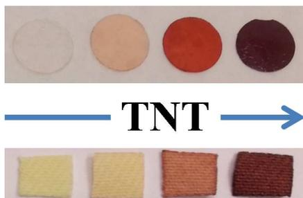
Visual detection of the explosive TNT with sensory polymer films and coated fibres
