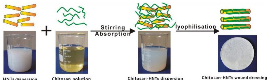
Figure 1 Schematic representation of the preparation of chitosan-HNTs composite sponges.
