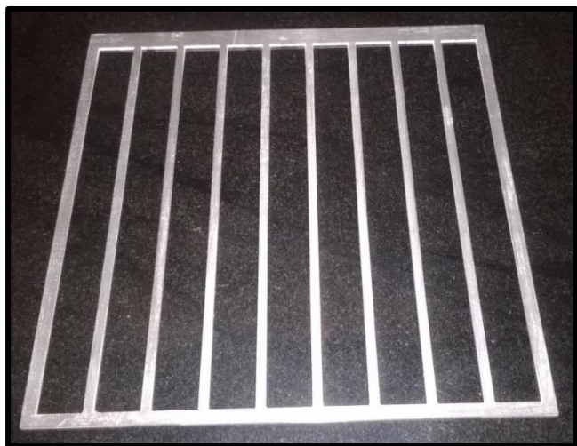
Fig. 4. The metallic (Ti) mask used to spray-deposit \text{TiO}_2 as compartments on the FTO substrate.
