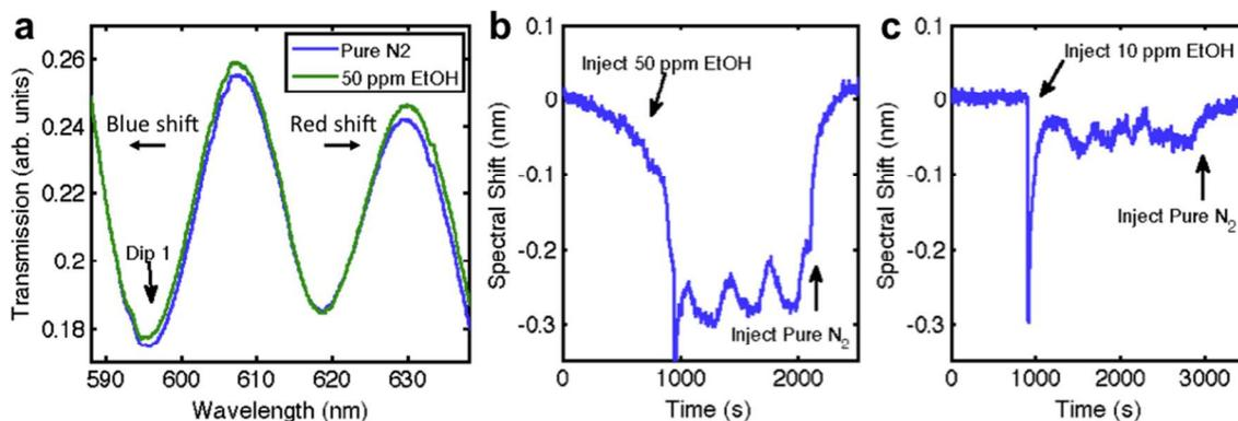
**Figure 4:** High-resolution transmission spectra and real-time sensing. (a) Using a higher-resolution spectrometer grating, higher sensitivity is obtained for both (b) 50 ppm ethanol vapor and (c) 10 ppm ethanol vapor. In this setup, the base noise level is nearing a  $\sim 1$  ppm detection limit. The pulsing likely comes from the syringe pump operating at near its lower limit.
