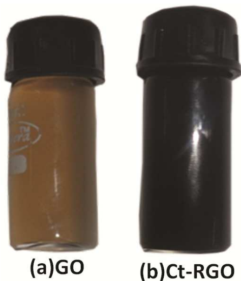
Figure 1: Photograph of (a) Graphene oxide (GO) and (b) Carrot reduced graphene oxide (Ct-RGO) in de-ionized water.
