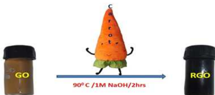
Scheme 1: Schematic representing the reduction of GO by Carrot
