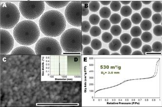
Fig. 1 Transmission and scanning electron microscopy of  $Fe_3O_4@MSN$  NPs (A-B, C respectively), the DLS size distribution (D), and N<sub>2</sub>-adsorption-desorption analysis (E).
