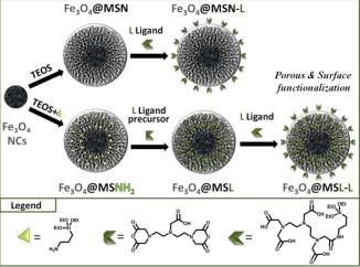
Scheme 2 Synthetic pathways to design ligand functionalized Fe<sub>3</sub>O<sub>4</sub>@MSN NPs.
