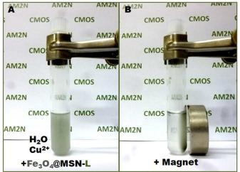
Fig. 2 Nanocontainers, before (A) and after magnetic separation of Fe₃O₄@MSN-L∩Cu<sup>2+</sup> NPs (B).
