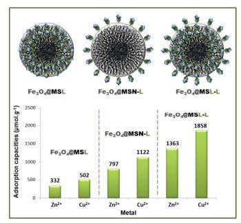
Fig. 4 Heavy metal removal capacities optimization of the various nanocontainers strategies.
