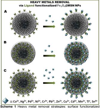
Scheme 1 Heavy metal removal strategies: surface functionalized Fe<sub>3</sub>O<sub>4</sub>@MSN NPs (A), the porous functionalized Fe<sub>3</sub>O<sub>4</sub>@MSN NPs (B), and surface/porous functionalized Fe<sub>3</sub>O<sub>4</sub>@MSN NPs (C).
