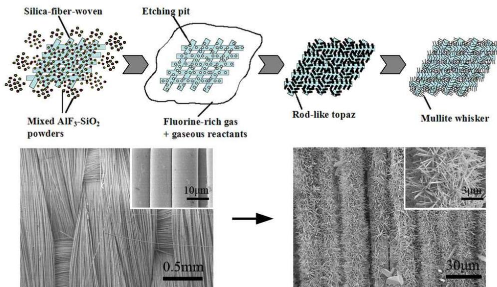
Hierarchical structural silica-fiber-woven/mullite-whiskers material prepared through surface etching and gas phase reaction was suitable for being applied as heat-sealing/insulation gasket at high temperature.
