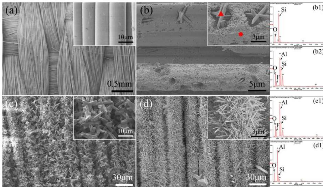
**Fig.1** SEM images and EDS results, (a) silica-fiber-woven as substrate, (b) the sample that formed at 800°C, (c) the sample that formed at 900°C, (d) the hierarchical structural silica-fiber-woven/mullite-whiskers material that formed at 1000°C, (b1) EDS result of the point that was marked with “●” in Fig.1b, (b2) EDS result of the point that was marked with “▲” in Fig.1b, (c1) EDS result of the rod-like grains in Fig.1c, and (d1) EDS result of the whiskers in Fig.1d.
