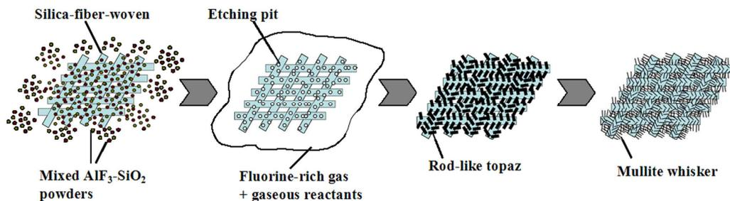
**Fig.4** Schematic diagram, structure forming process of the hierarchical structural silica-fiber-woven/mullite-whiskers material.
