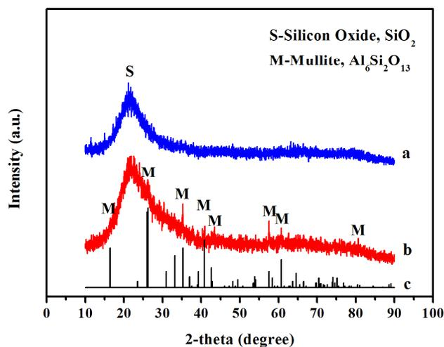
**Fig.2** XRD patterns of the silica-fiber-woven (a) and the hierarchical structural silica-fiber-woven/mullite-whiskers material (b), and the standard pattern of mullite phase (PDF#15-0776) (c).
