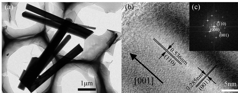
**Fig.3** TEM images (a, b) of the mullite whiskers which were peeled off from the hierarchical structural silica-fiber-woven/mullite-whiskers material, and (c) was the mullite lattice's reciprocal lattice pattern by fast Fourier transform (FFT).
